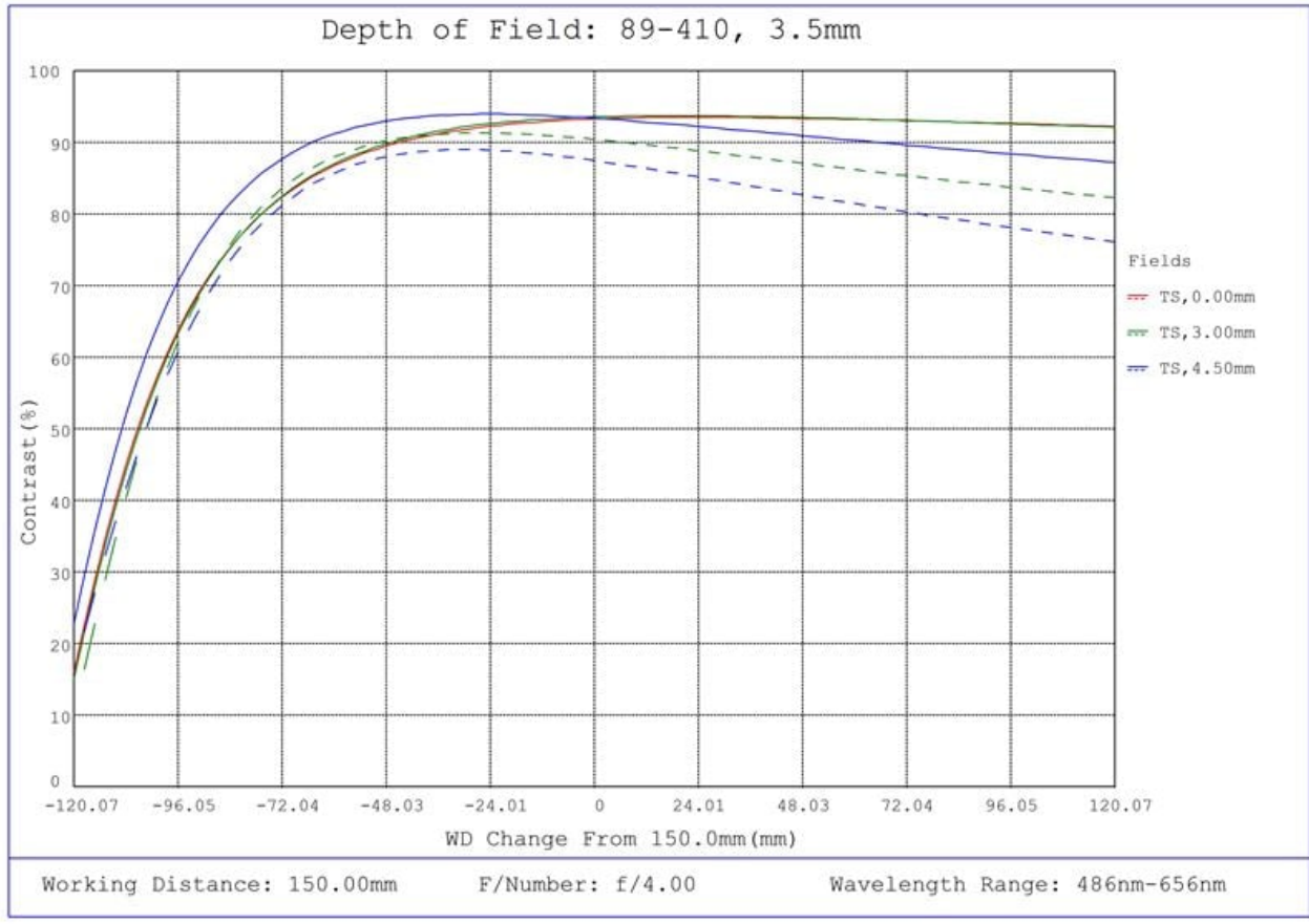
#89-410, 3.5mm C Series Fixed Focal Length Lens, Depth of Field Plot, 150mm Working Distance, f4
