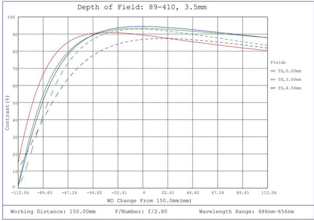
#89-410, 3.5mm C Series Fixed Focal Length Lens, Depth of Field Plot, 150mm Working Distance, f2.8
