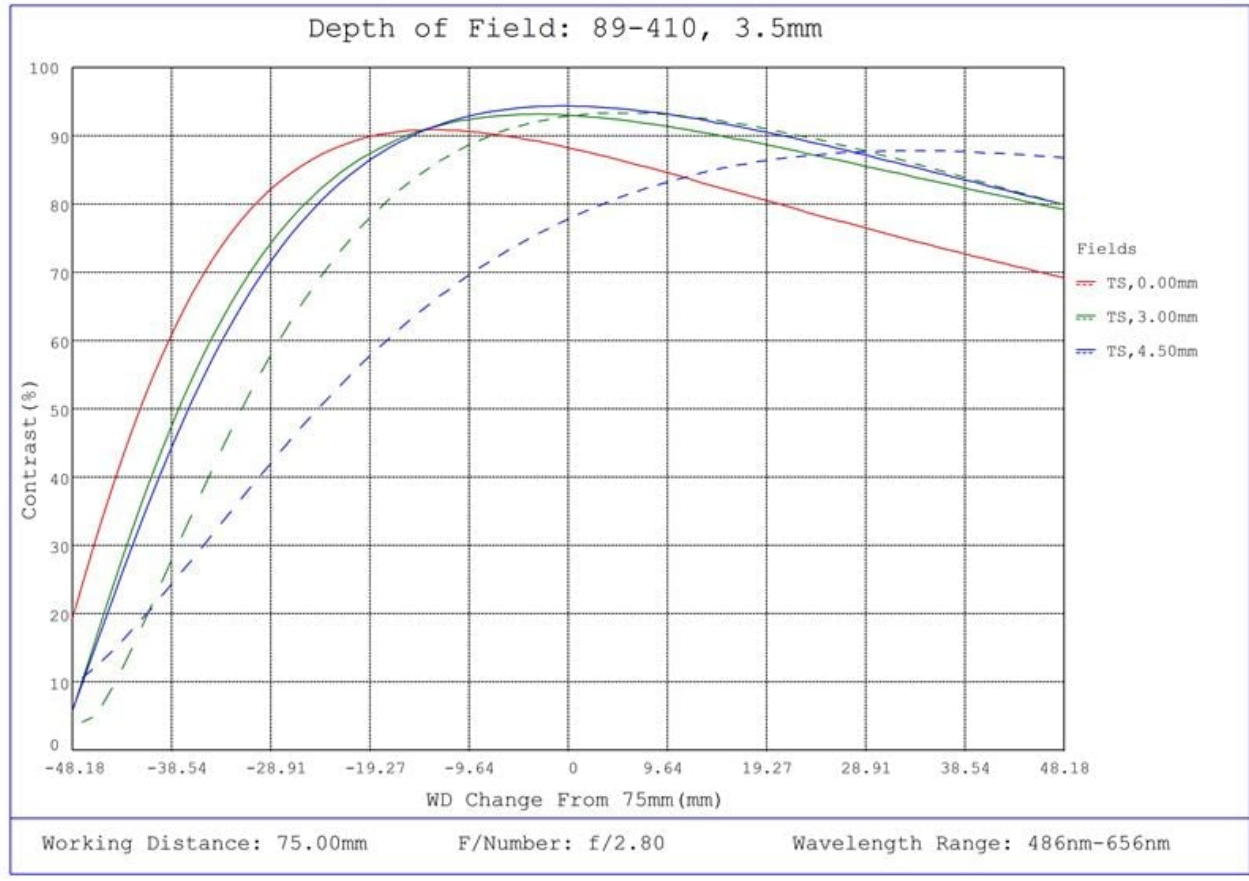
#89-410, 3.5mm C Series Fixed Focal Length Lens, Depth of Field Plot, 75mm Working Distance, f2.8
