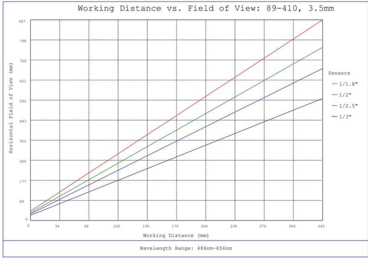
#89-410, 3.5mm C Series Fixed Focal Length Lens, Working Distance versus Field of View Plot
