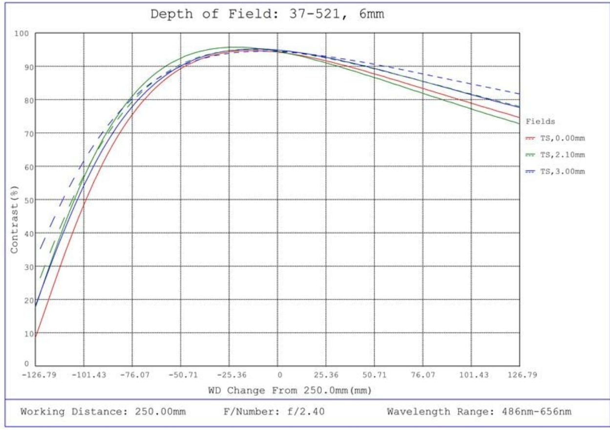
#37-521, 6mm FL, Liquid Lens M12 Lens, Depth of Field Plot, 250mm Working Distance, f2.4
