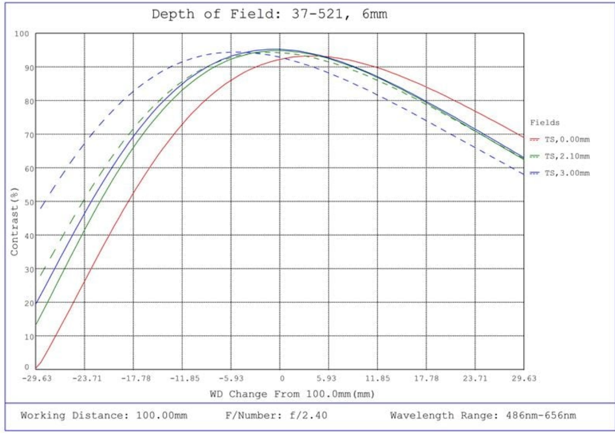
#37-521, 6mm FL, Liquid Lens M12 Lens, Depth of Field Plot, 100mm Working Distance, f2.4
