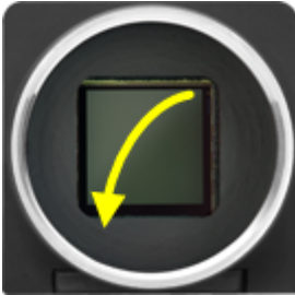
Fig. 15: Cleaning fixed filter glasses (1)
