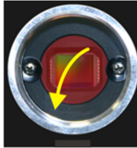
Fig. 16: Cleaning fixed filter glasses (2)
